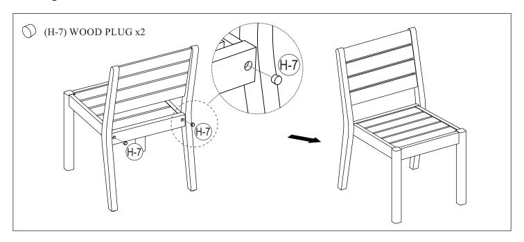
Turn chair upright, Insert Wood Plugs (H-7) into bolt holes in Backrest (A) until roughly flush. If needed, cover plugs with a padded surface (such as cardboard) and gently tap with a hammer or mallet (not provided). Assembly is now complete and the chair is ready for use.
