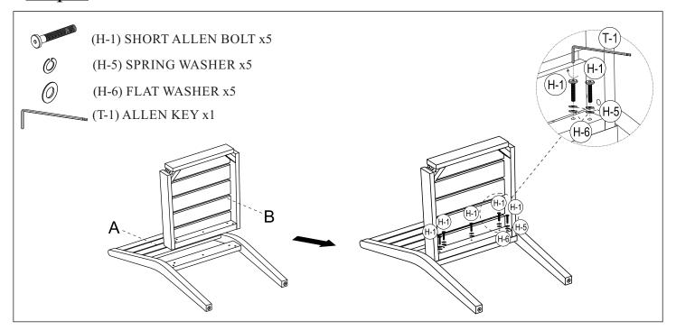
Place Backrest (A) upside down on a padded non - marring surface. Secure Seat Panel (B) to Backrest (A) with Allen Bolts (H-1). Spring Washers (H-5) and Flat Washers (H-6) using provided Allen Key (T-1), stacking the hardware in the order as shown. Engage all bolts first, then fully tighten. DO NOT OVER TIGHTEN.
