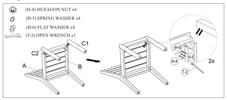
Place Backrest (A) down onto a padded, non-marring surface. Insert bolts in Left Front Leg (C1) and Right Front Leg (C2) into front corners. Secure with Hexagon Nuts (H-4), Spring Washers (H-5) and Flat Washers (H-6) using provided Open Wrench (T-2), stacking the hardware in the order as shown. Fully tighten, but do not over tighten.
